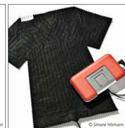
Electronic control for heating on demand
